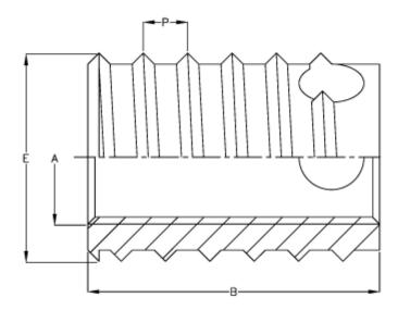
Female thread A = M12 Length B = 22 Male thread E = 16.0 Min hole depth blind hole = 26 Thread pitch P = 1.75
